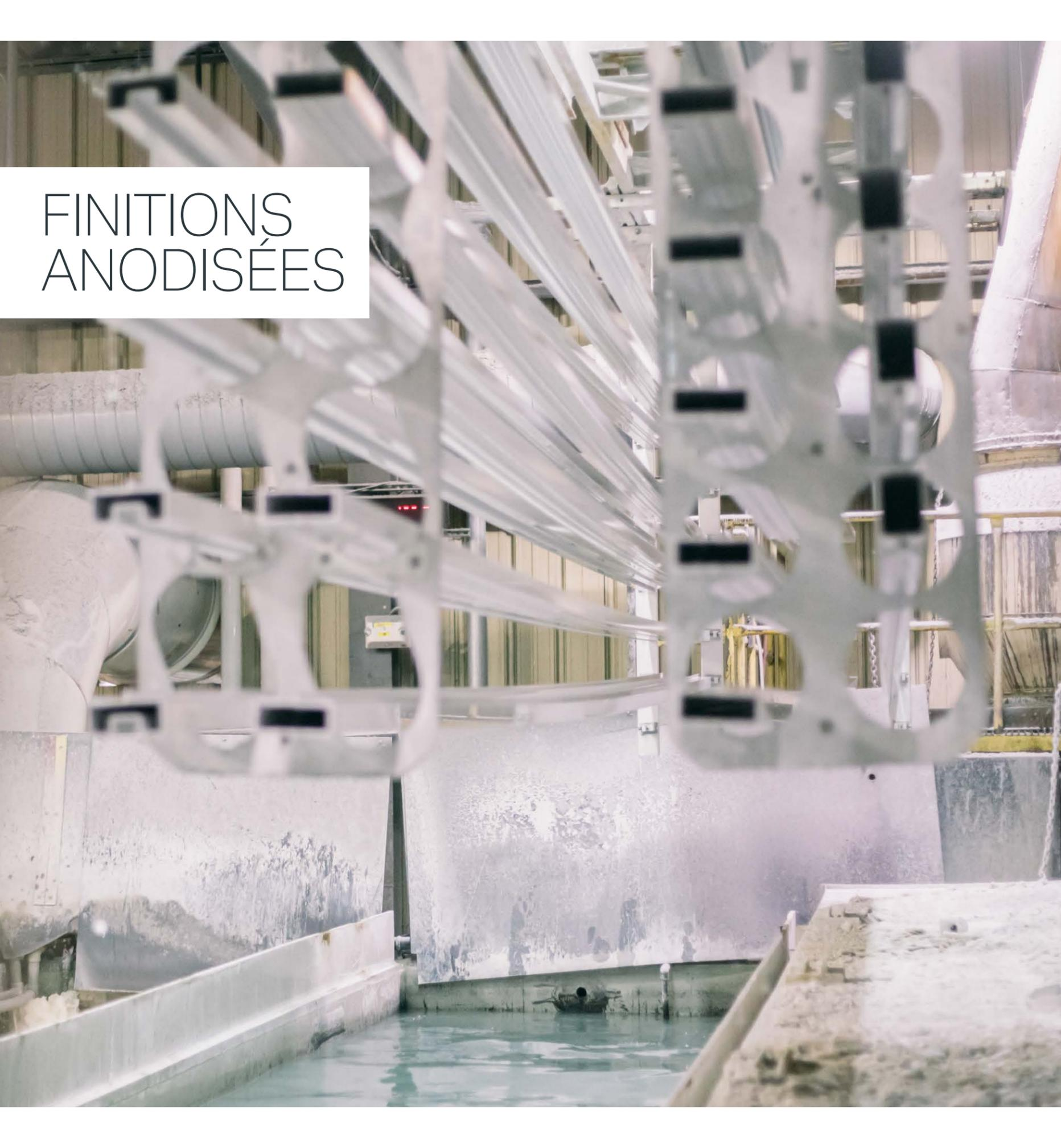
The image shows a large industrial anodizing plant. In the foreground, a metal rack with a repeating circular pattern is out of focus. Behind it, several long, parallel metal racks are suspended over a large tank containing a light blue electrolyte solution. The racks are filled with aluminum parts. The background shows the complex structure of the facility, including pipes and structural beams.
